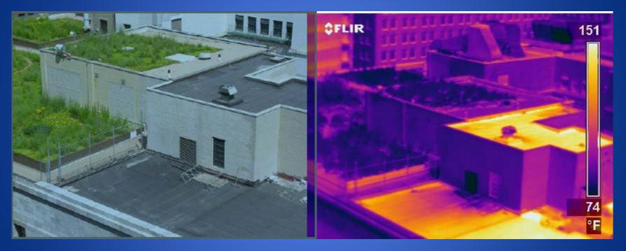
Heat sensing pictures illustrate the major temperature difference between green roofing on
